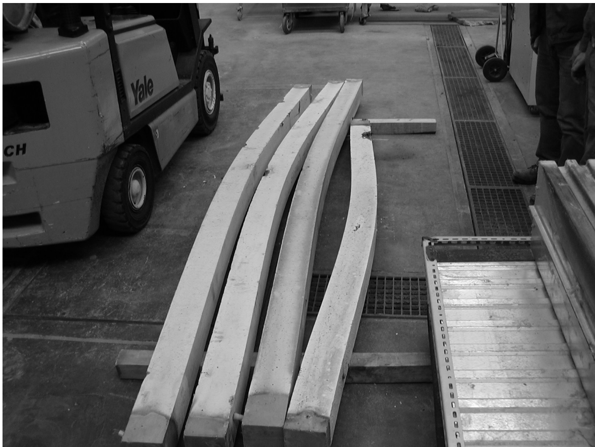
Figure 9 - Some of the columns after fire exposure.
