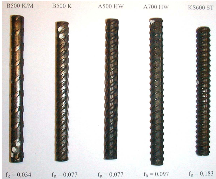
Figure 3 Specimens used in relative rib area measurement (testing year 1999).
