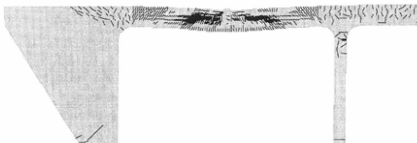
Figure 9 - Detailed crack patterns at final loading state predicted by Atena [20]. The cracks illustrated are of widths > 0,1 mm].
