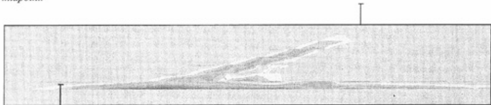
b) Concentration of principal tensile strains, illustrating the horizontal and diagonal crack pattern at a deflection of 30mm at midpoint.
