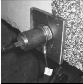
Figure 4 – Wedge anchor, load cell and anchor plate.
