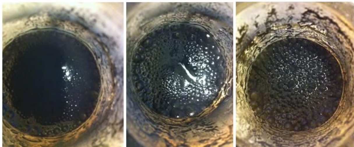
Figure 2 – Evolution of foaming in 40 mm diameter FI test container of high Carbon fly ash in figure 1 (Ollendorff 2011)
