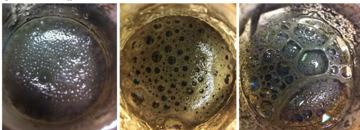
Figure 3 – Varying foam structures at stable foaming of (from left) ash No. 3, 2 and 1 in figure 1 (Ollendorff 2011)
