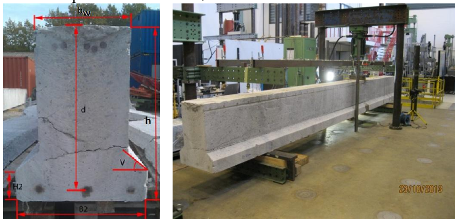
Figure 1: Left: Specimen geometry and reinforcement ratio in one of the tested beams. bw = 0.39 m, B2 = 0.60 m, H2 = 0.13 m, h = 0.74 m, V = 45^\circ and d = 0.68 m. Right: Asymmetrical three point bending test rig with the length of 5.6 m between supports.
