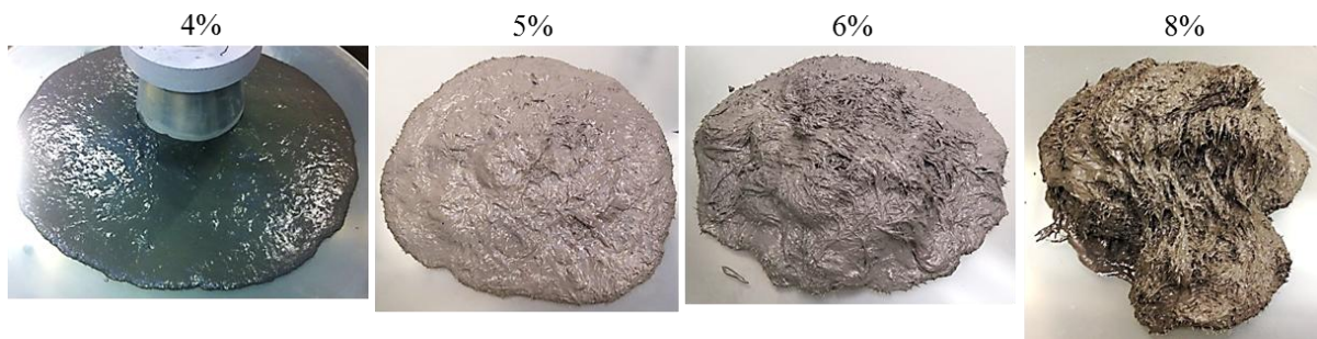
Figure 1 – Slump test of UHPFRC concrete for different fibre volume fractions.
