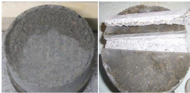
Figure 2 - Surface with the ITZ of granite and shotcrete (left.) The half-moon shaped area on the upper part of the granite core shows the positions of shotcrete residuals. A slice containing granite core and epoxy with the interfacial zone just in between is shown in the upper part of the right photo.
