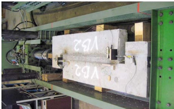
Figure 3 – Test bench (left) with test specimen and load-deformation relation for three different joint designs (U-stirrups and alternatives in a smooth joint) /Nielsen and Nordkvist, 2014/
