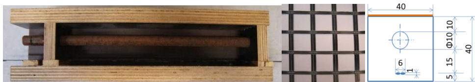
Figure 1 Image of the casting mould (left), the carbon fiber mesh anode (middle) and the dimension of specimen (right).
