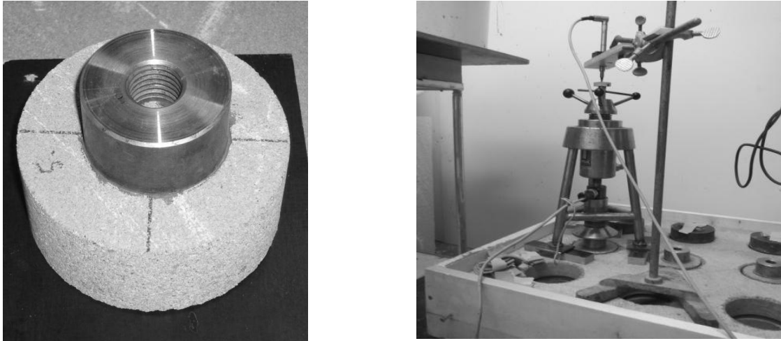
Figure 2 – Core of concrete adhered to a coupling steel disc. Pull out tester with load cell and strain gauge (LVDT). From (Bryne et al., 2013, 2014).
