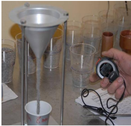
Figure 2 – Flow time measurements of the same fractions as in Figure 1.
