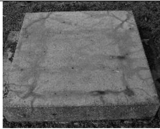
b) Surface of concrete exposed to natural weathering + deicing salts
