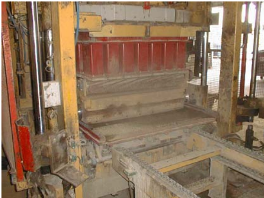
Figure 4 – Compaction of paving stones.
