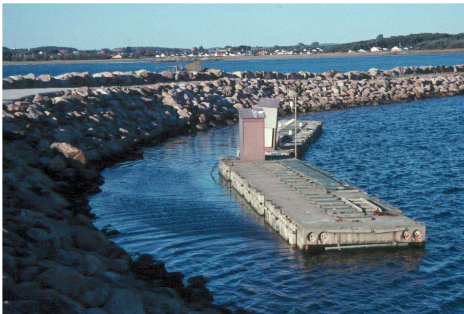
Figure 1 – The field station in the harbour of Träslövsläge. Concrete slabs are hanging from both sides of the floating pontoons.
