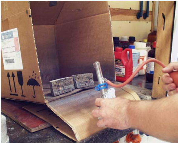
Figure 3.5 - Point-one M silver nitrate solution sprayed to the specimen [4].
