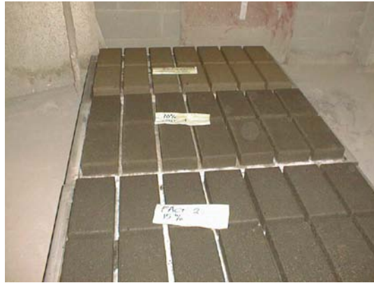
Figure 8 – Comparison of the three different paving stone colors (from back: 0, 10 and 15% residue).
