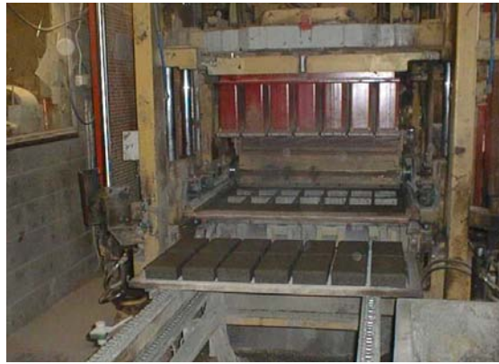
Figure 5 – Tray of paving stones moving out of compaction machine in factory.
