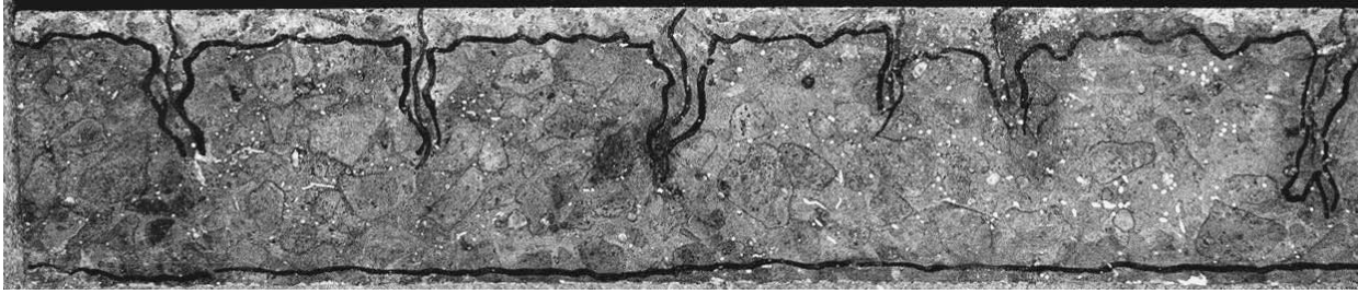
Figure 2 - Chloride exposed specimen after UV-test. Concrete SA-ZP. Exposure time 13 months. Load level 3.6 kNm. The beam contains 7 mechanically induced cracks, crack width between 0.07 and 0.28 mm (one crack is not included on Figure 2). Overall average crack width 0.17 mm. Beam size in vertical direction 100 mm. Thick, mostly horizontal lines indicate the boundary found by the UV-test. Thinner, vertical lines indicate the visible, mechanically induced cracks.
