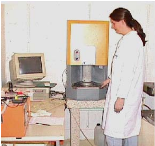
Figure 3 – ICT machine to simulate paving block manufacturing in a laboratory.
