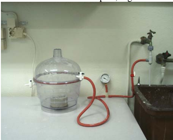
Figure 3.1 - The surface-dry specimens were placed in a vacuum container to a pressure in the range of 1-5 kPa within a few minutes.
