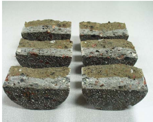
Figure 3.6 – Test specimen after preparation for chloride penetration measurement [4].
