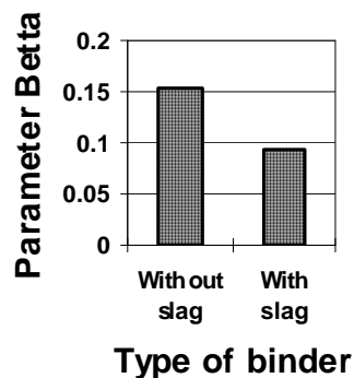
Figure 4 - Effect of type of binder on \beta . Curing time in fresh water were 1, 7, 28 and 365 days before the specimens were exposed to sea-water. The results reflects the difference in D for companion specimens stored in sea-water and specimens stored in fresh water in periods given above + 35 days in sea-water to get a chloride profile to analyse. [16]
