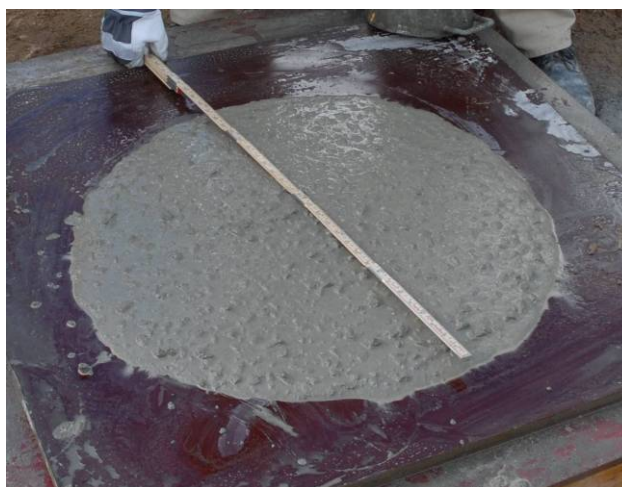
Figure 13: Slump flow of tested SCC, measuring approximately 700 mm.
