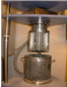
Figure 2 – The coaxial cylinder ConTec viscometer 4 controlled by computer software.
