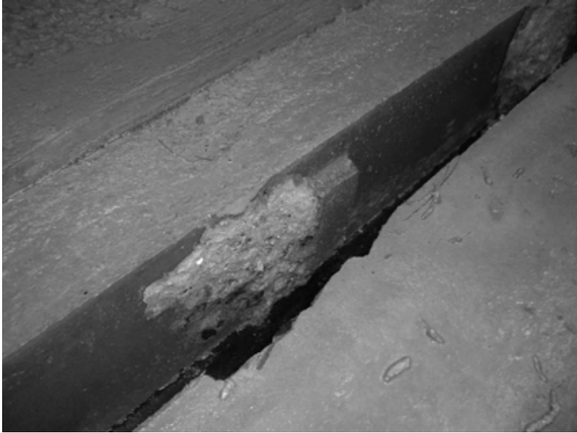
Figure 10 – Failure in concrete element in joint detail 8, test no. 8.1, CRC JointCast, no reinforcement, three indentations 90 x 40 mm
