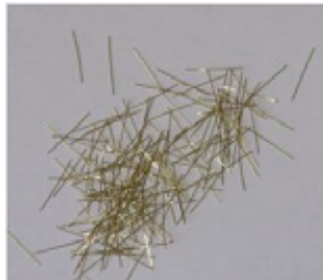
Figure 1 – Bekaert OL13/.16 Straight high carbon steel fibers.
