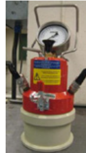
Figure 3 – Pressure-type air meter used for measuring the air-void content and the density of fresh mortar in our study.
