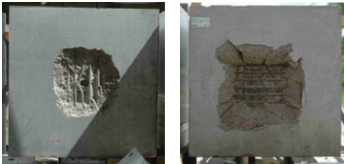
Figure 13. Post-test photos of front and back faces of target from test no. 2004-20 [10], which corresponds to the simulation identity FAE5-01.
