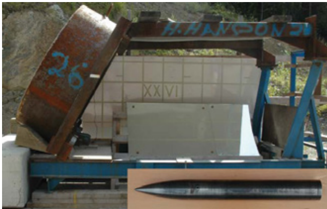
Figure 1. Experimental set-up for oblique target tests [10], with background and mirror for high-speed filming of the horizontal and vertical projections of penetrator shown. The insert show the external design of the penetrator.
