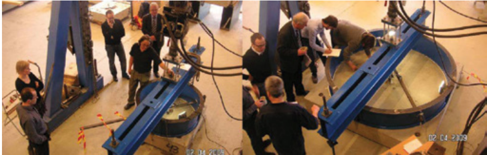
Figure 4 – Test set-up: support ring with radius 0.55 m (left) and with radius 1.1 m (right).
