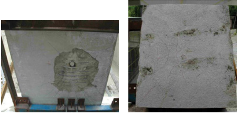
Figure 16. Post-test photos of front and back faces of target from test no. 2004-24 [10], which corresponds to the simulation identity FEA6-01.
