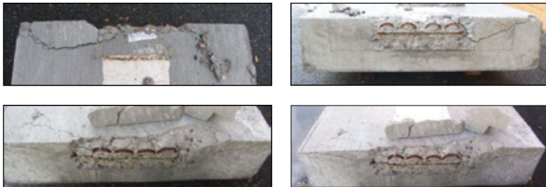
Figure 14 – Photos of shear key type 1 after failure in the concrete covering layer.
