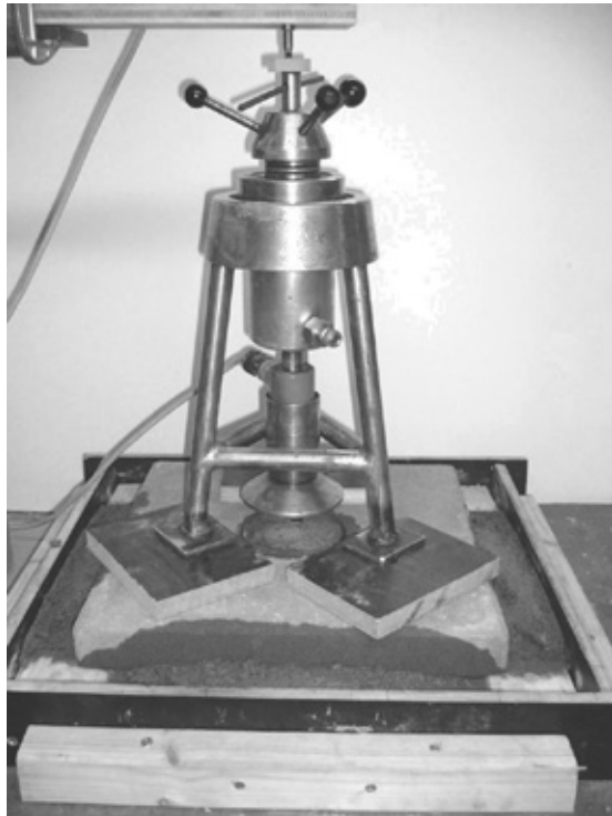
Figure 6 – Precast concrete slab on top of newly cast concrete and bond strength testing device with load cell and strain gauge (LVDT).
