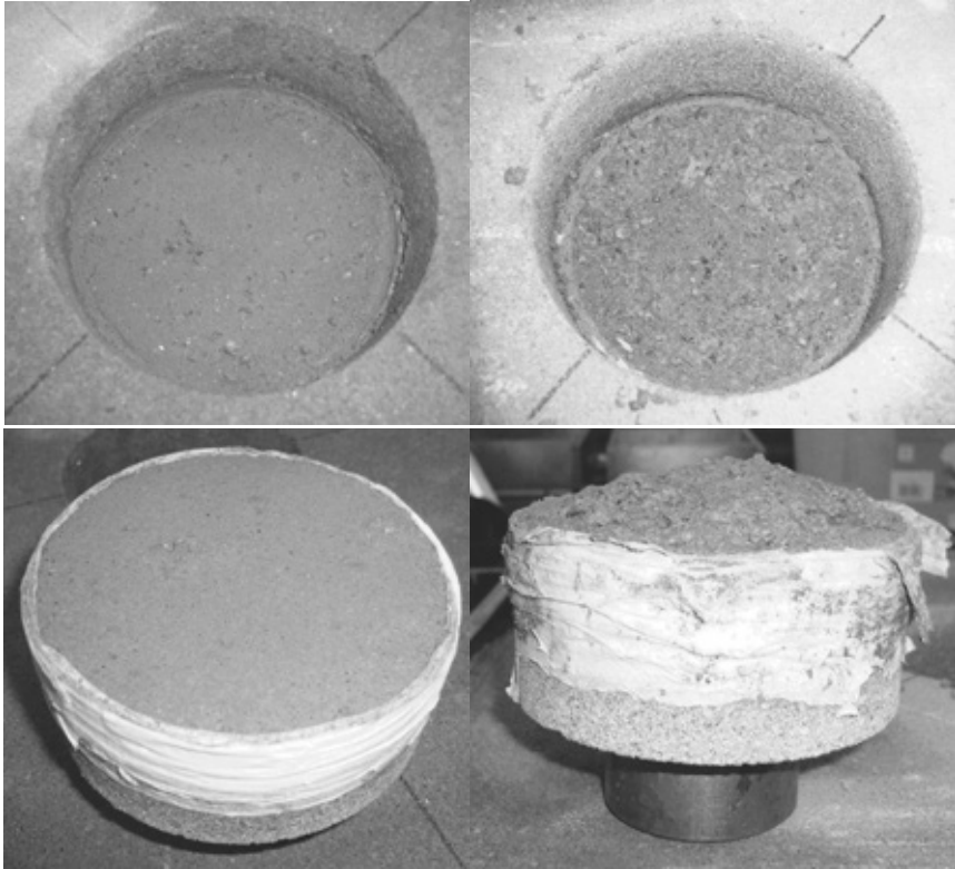
Figure 9 – Typical failure surfaces, delamination (left) and tensile, material failure (right).
