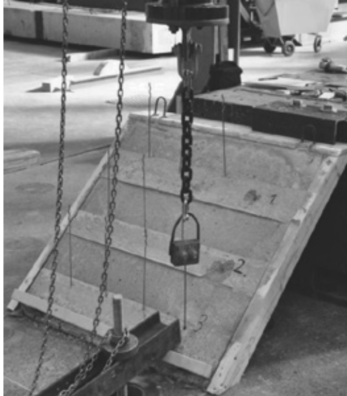
Figure 6 – Principle of 45 degree tensile strength tests.
