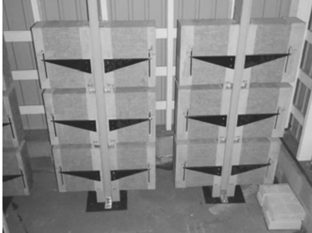
Figure 5 – Long-term test specimens were mounted on special racks inside a well-ventilated shelter.
