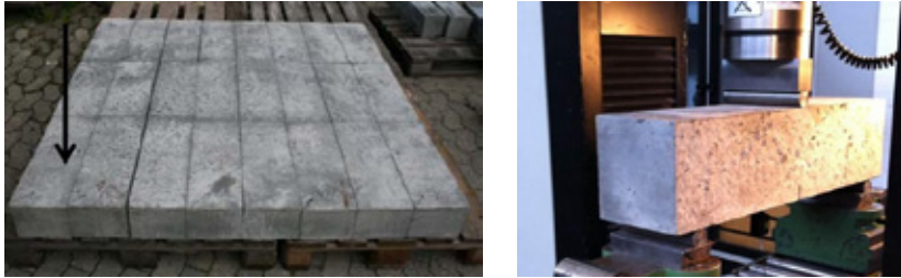
Figure 3 – Left: The slab saw cut into 24 beam specimens. Right: Three-point bending test.
