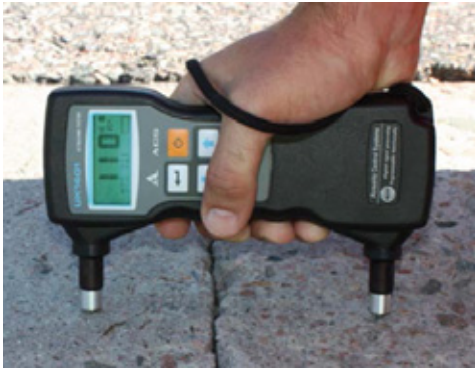
Figure 4 – Surfer in practice (Displaying crack depth d = 110\text{ mm} ) [9].
