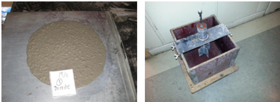
Figure 7 – Slump-flow test (left) and the Portable Vane, equipment for measuring torque (right).
