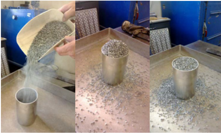
Figure 1 – Testing of loose particle packing.
