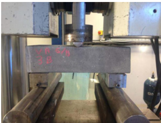
Figure 4. A concrete test beam made with Energetically Modified Cement (EMC) undergoing RILEM 3-point bending [23] at Complab, LTU.
