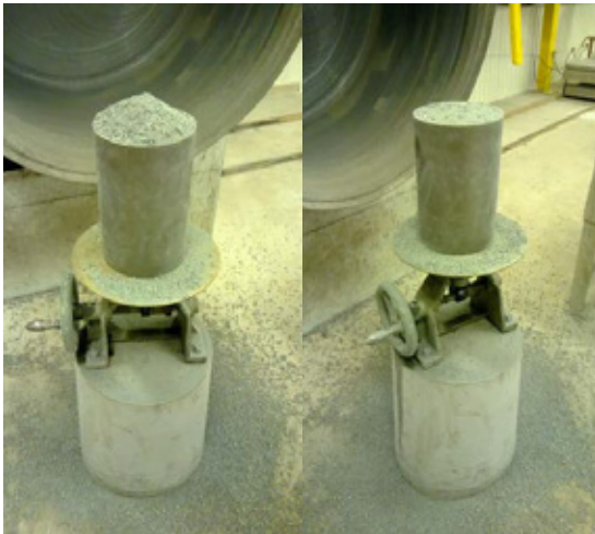
Figure 2 – Testing of compressive particle packing.
