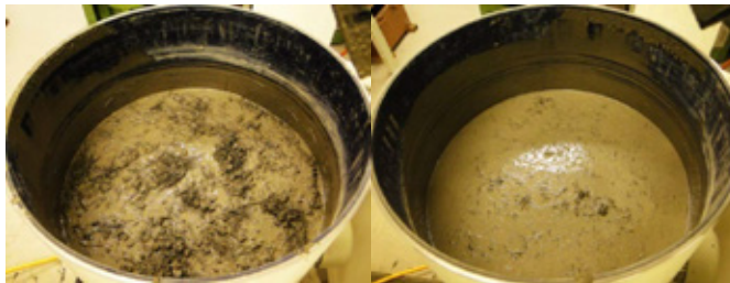
Figure 9 - In the left hand side, concrete with fiber content of 2.5% after 7 minutes of mixing is shown. Right hand side shows the broken fibres after extended mixing time.
