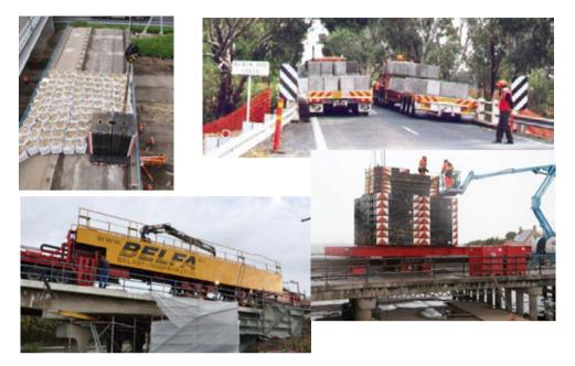
Fig.5: Different setups proof loading slab viaducts
