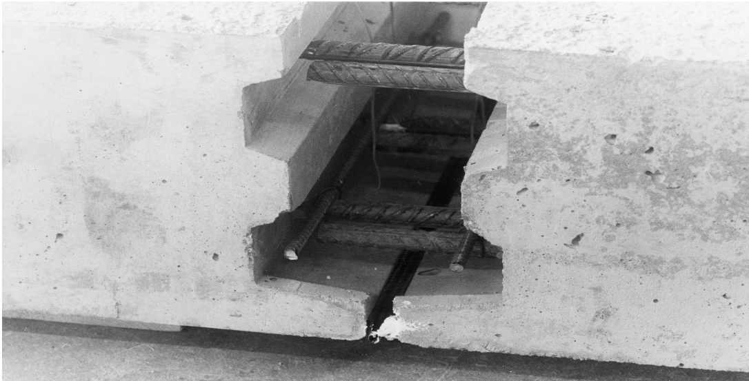
Figure 4. An example of result from combination of materials development and research in structural engineering; an innovative new joint concept for structural joints between concrete members.
