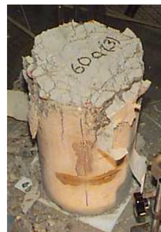
Fig 3. Unconfined specimen 60a-3t (with teflon) after failure. Vertical cracks.
