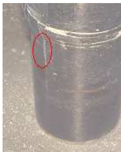
Fig.7.a. Specimen 20c1L1C-1t after failure. Detection of the slight debonding at the overlap edge.
