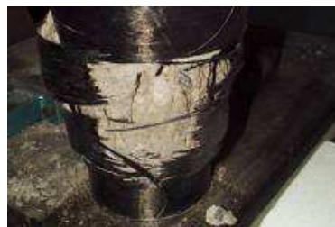
Figure 2.b. Shear cone failure of specimen with 100 mm overlap length. (Without teflon)
