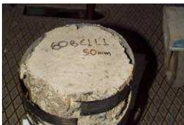
Figure 2.a. Debonding of specimen with 50 mm overlap length and use of teflon.
