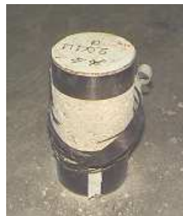
Fig. 7.c. Specimen 20c1L1-3t after failure.
