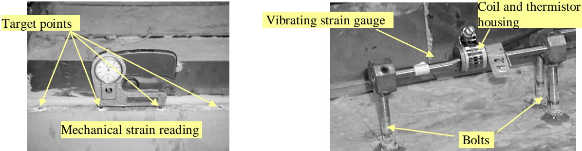
Figure 4 – Strain measurement devices used in the study. A mechanical strain reading device to the left (Staeger) and a Vibrating Wire Strain Gauge (VSG) to the right.
