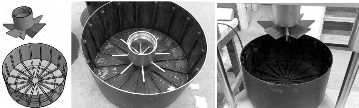
Figure 1 – The Coplate 5 system – Mark III. All interior of the bucket (black) as well as the whole top unit (grey) consists of protruding vanes to avoid slippage. Fig. 2 shows the relative position of these two units during a rheological test.
