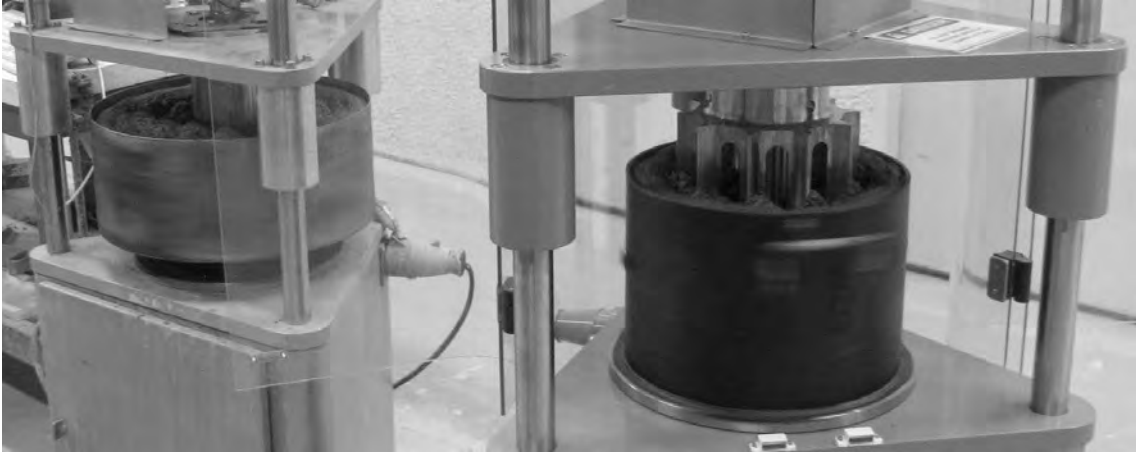
Figure 4 – Simultaneous testing of the Coplate 5 system (to the left) and of the coaxial cylinders system (to the right).
