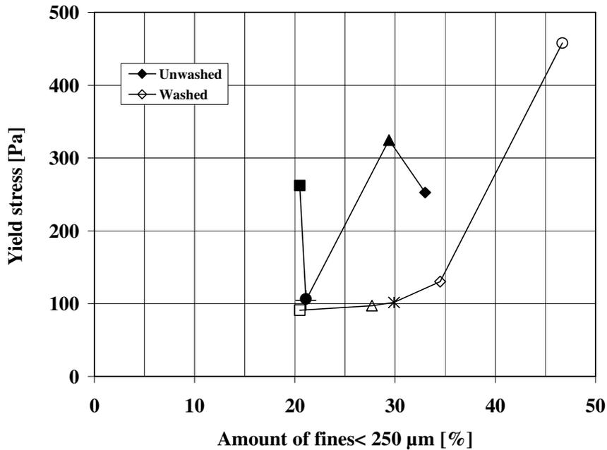
Figure 5 – Yield stress of mortars as a function of the amount of fines < 250 μm in the washed and unwashed aggregates. Filled and open symbols represents unwashed and washed aggregates, respectively. \* = C18W, + = C3; grading = N1.
