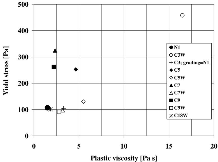
Figure 4 - Rheological properties of mortars with unwashed and washed (W) aggregate.
