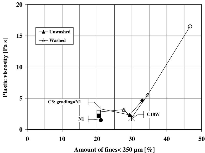
Figure 6 – Plastic viscosity of mortars as a function of the amount of fines < 250 μm in the washed and unwashed aggregates. Filled and open symbols represents unwashed and washed aggregates, respectively. \* = C18W, + = C3; grading = N1.
