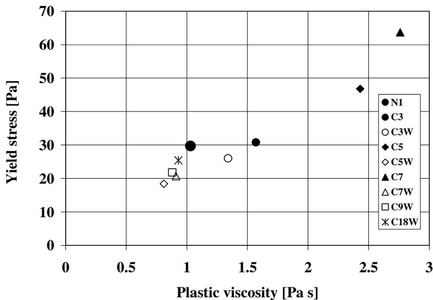
*Figure 7 - Yield stress and plastic viscosity of micromortars containing unwashed and washed (W) aggregate fines.*
