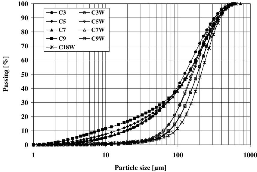
Figure 3 - Particle size distribution of the fine particles prior to and after washing.
