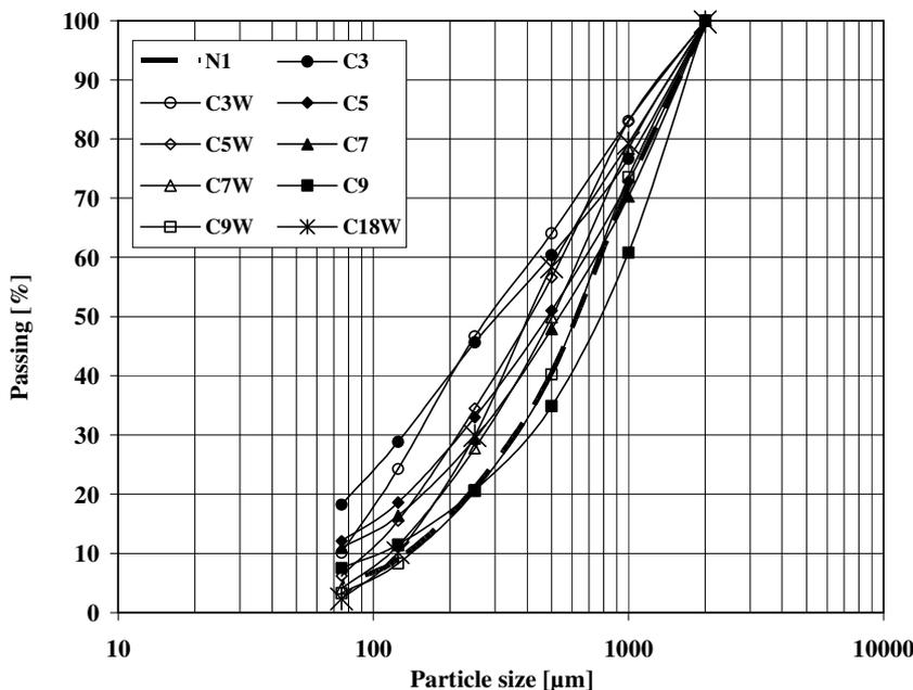
Figure 2 - Particle size distribution of unwashed and washed (W) aggregates.
