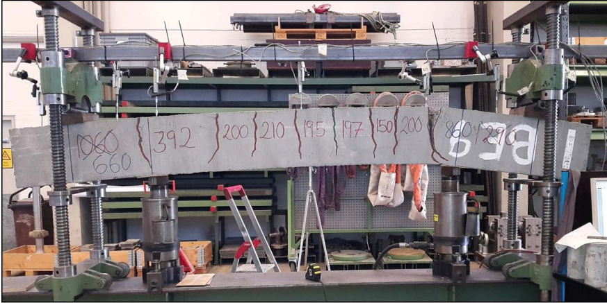
Figure 1 – Test setup with beam Q2 after failure [2].
