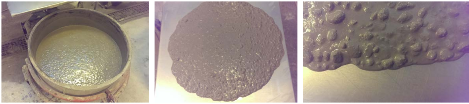
Figure 2 – Concrete is clearly segregated in the container (left). Some segregation visible at slump flow test (center). Stones are present at the edge of concrete from slump flow (right)
