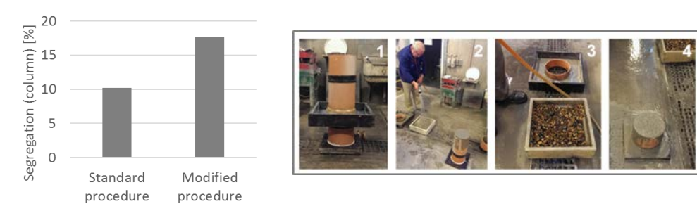
Figure 3 – Segregation with standard procedure and a modified procedure with 2 sec vibration for the same concrete mix design (left). Measurement of column segregation in steps (right)
