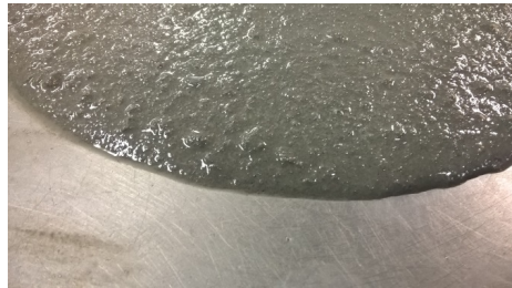
Figure 2 – Haegermann flow of concrete during laboratory development.
