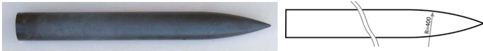
Figure 2 – Model projectile with 50 mm diameter, 450 mm length and 400 mm ogive radius [1,2]. Definition of the nose section radius is shown to the right.
