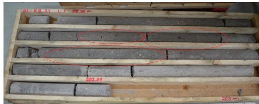
Figure 3 – Cored concrete samples taken from in-situ demonstration.
