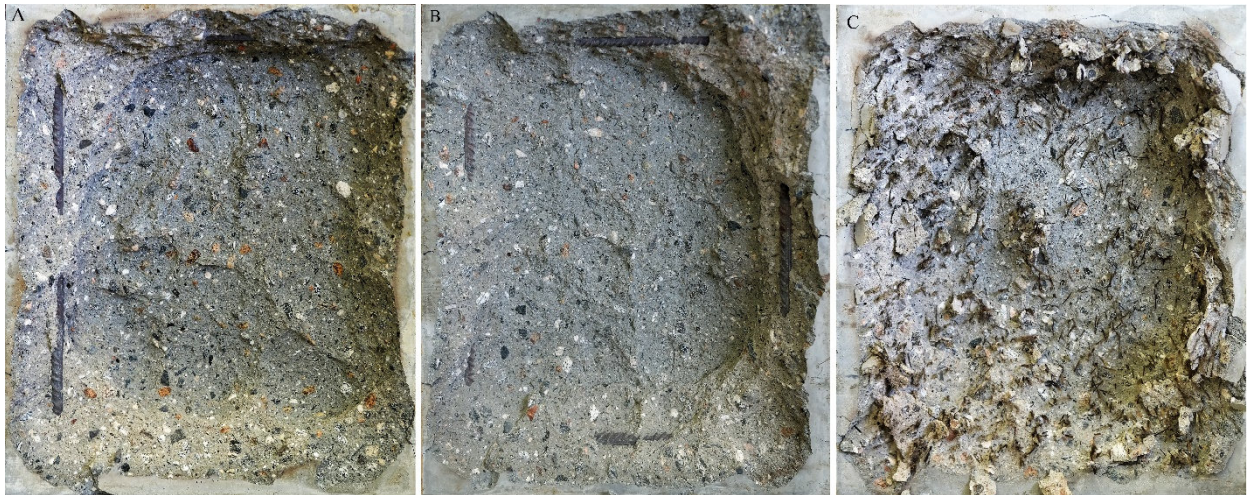
Figure 9 - The concrete samples after exposure to fire. (A) represents MIX-0-R, (B) MIX-0.5-C and (C) MIX-0.5-M.
