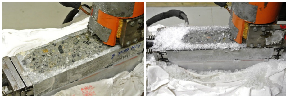
Figure 10 – Photos of concrete surface during two types of test: (a) sliding; (b) sliding-spallation.
