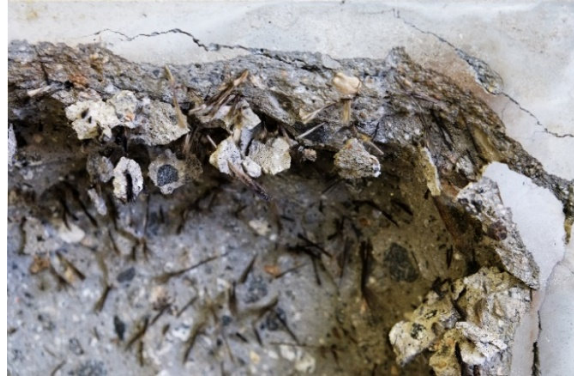
Figure 10 - The concrete pieces are still connected to the main specimen via macro fibres after fire exposure.
