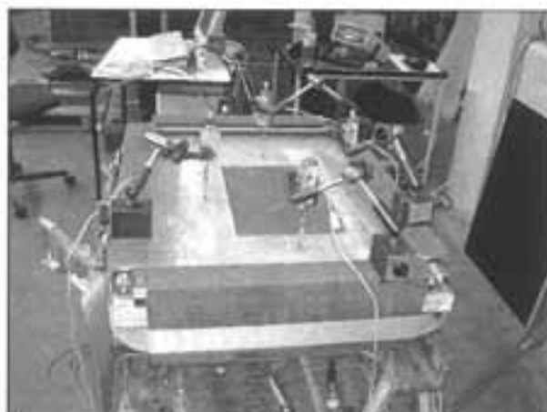
Figure 2 – Down-sized testing of concrete panel with a window plate /2/.
