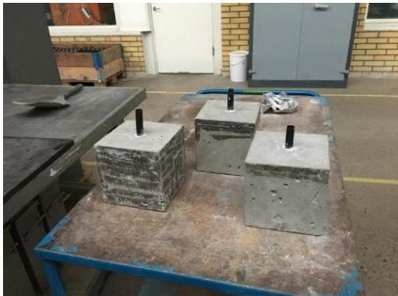
*Figure 4 – The investigated concrete cubes resting on a carriage before measurement of their respective weight.*
