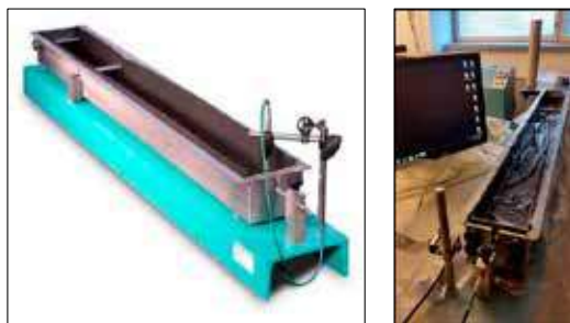
Figure 5. Early-age deformation test with the Schleibinger Bending-Drain – rig.
