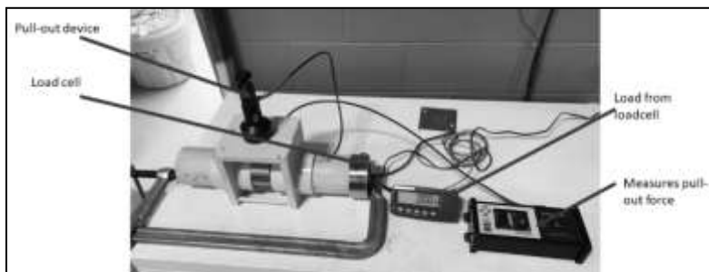
Figure 5 – Simple design concept for double-shear adhesion tests.
