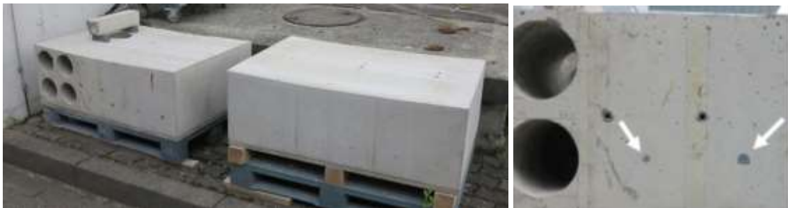
Figure 2 – Concrete blocks (left) with sensors (right)
