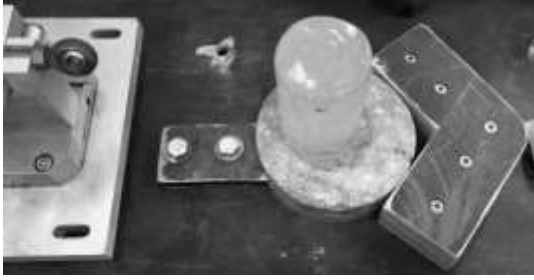
Figure 4 – Test set-up for direct shear tests, using a modified friction table.
