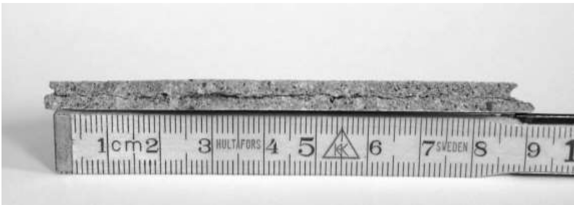
Crack in the center of w/c ratio 0.65 specimen stored in 3% NaCl solution for 19 days prior to test at -10^{\circ}\text{C} , bath salt concentration 14.4%. (Two views). Crack is assumed to be due to ice crystals growing at the centre of the specimen, where the salt concentration was at the lowest.
