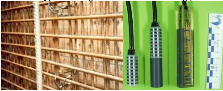
Figure 1 – MRE and MTP (left), Sensor installation in a structure (right)
