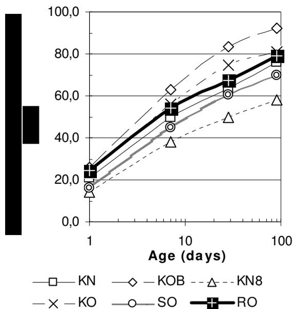
Figure 3 – Concrete strength development.
