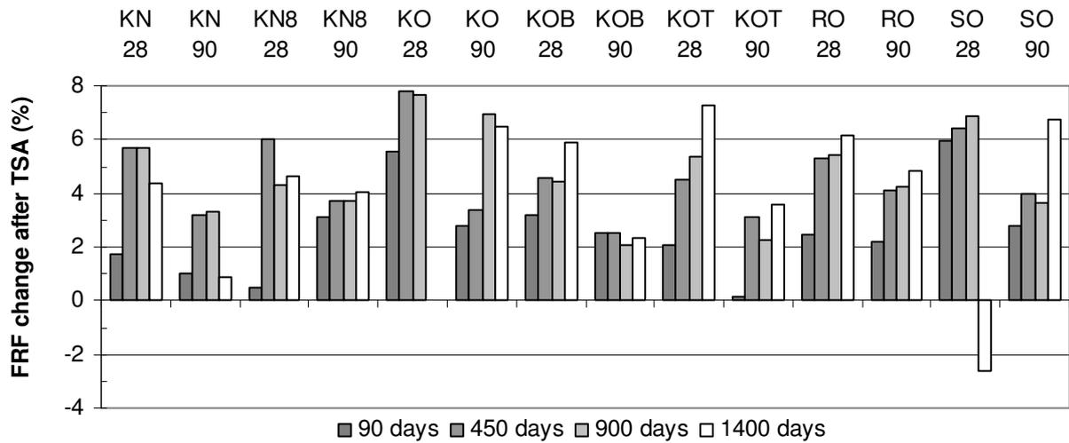
Figure 7 –FRF change after 1400 days of exposure in 18 g/l of sodium sulphate in distilled water at 5 °C.
