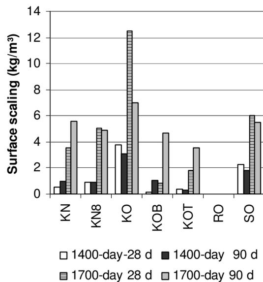
Figure 10 –Scaling at 1400 and 1700 days.
