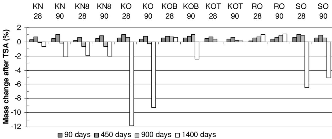
Figure 9 –Mass change after 1400 days of exposure in 18 g/l of sodium sulphate in distilled water at 5 °C.
