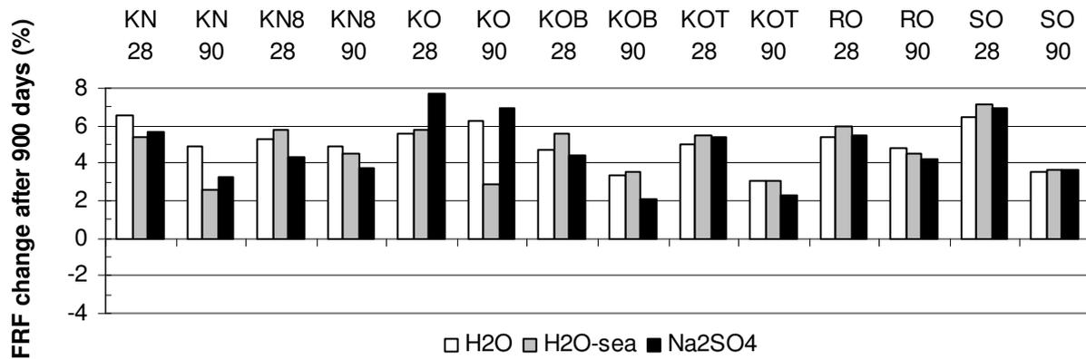
Figure 4 – FRF change after 900 days at 5 °C. FRF = fundamental resonance frequency.
