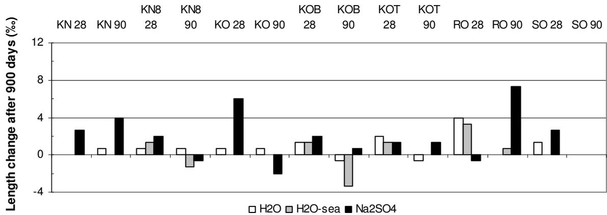
Figure 5 – Change of length after 900 days of exposure at 5 °C.
