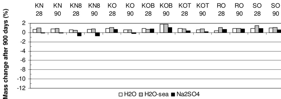
Figure 6 – Change of mass after 900 days of exposure at 5 °C.
