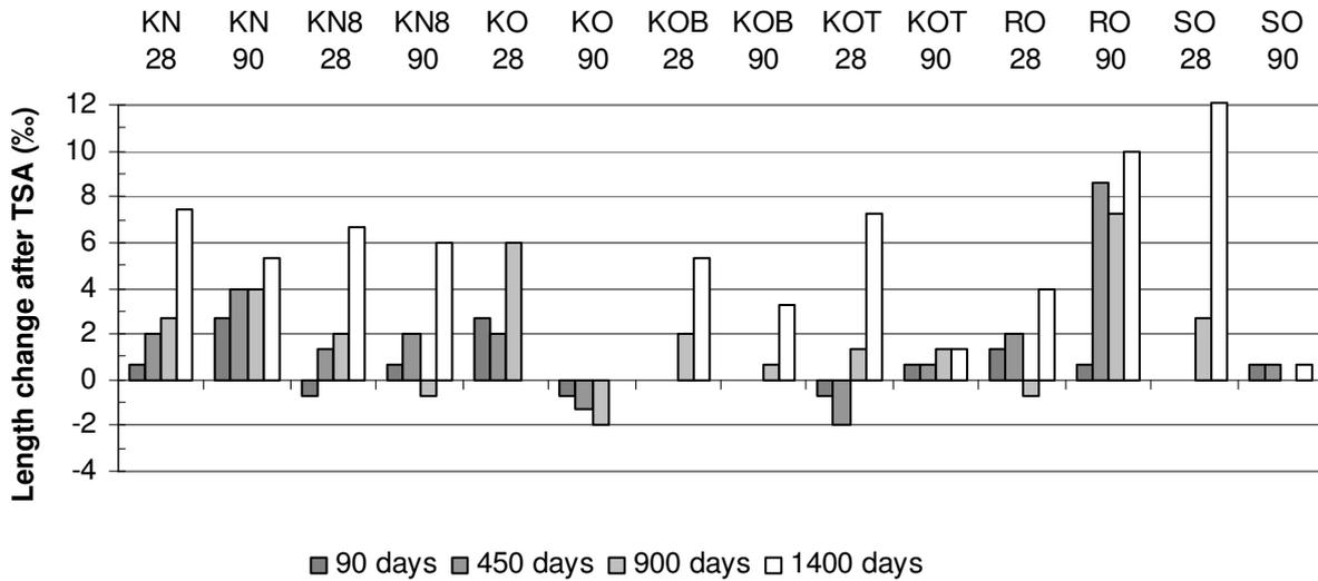
Figure 8 –Length change after 1400 days of exposure in 18 g/l of sodium sulphate in distilled water at 5 °C.
