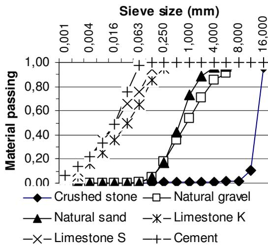
Figure 1 – Material grading curves.
