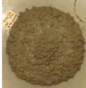
Figure 16 – 0.5 % fibre, Slump-flow = 450 mm
