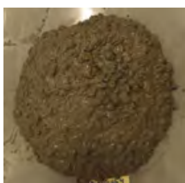
Figure 13 – 0.5 % fibre, Slump-flow =430 mm
