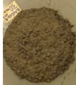
Figure 17 – 1.0 % fibre, Slump-flow = 390 mm
