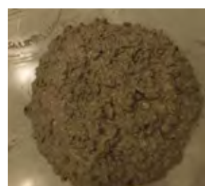
Figure 14 – 1.0 % fibre, Slump-flow =390 mm
