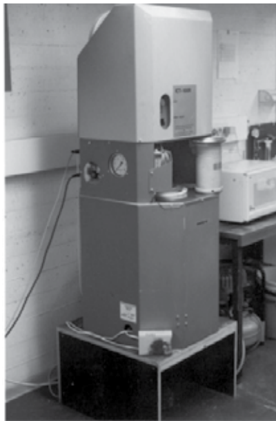
Figure 1 - The gyratory compactor used for this work
