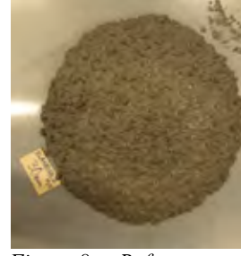
Figure 8 – Reference concrete, 30 min after water, Slump-flow =510 mm
