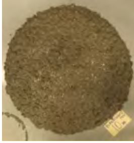
Figure 6 – Reference concrete, 10 min after water, Slump-flow=550 mm
