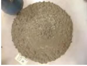
Figure 9 – Without fibre, Slump-flow=540 mm
