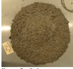
Figure 7 – Reference concrete, 20 min after water, Slump-flow =520 mm
