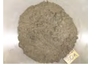
Figure 11 – 0.5 % fibre, Slump-flow =440 mm
