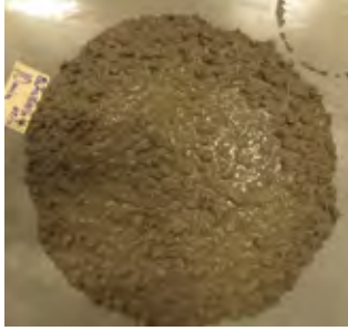
Figure 15 – 0 % fibre, Slump-flow = 520 mm
