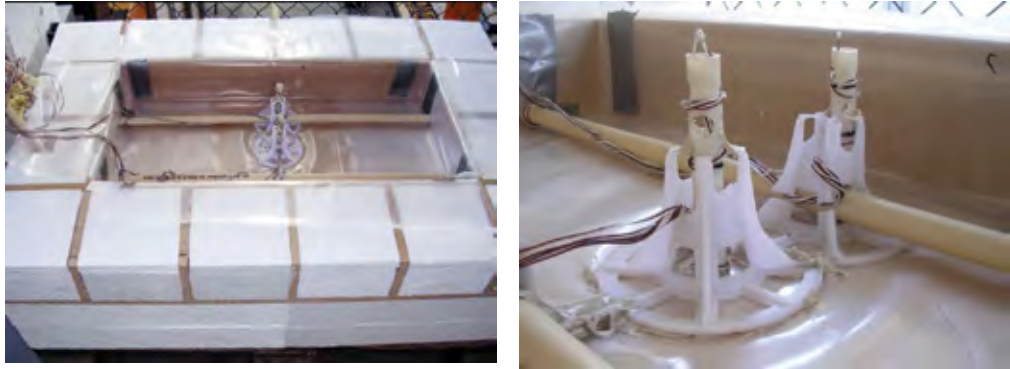
Figure 1. Mould (batch 1) with cast in heating pipes and console for thermo element.
