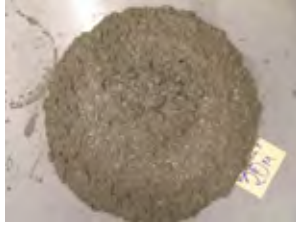
Figure 10 – 0.25 % fibre, Slump-flow =440 mm
