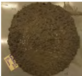
Figure 12 – 0 % fibre, Slump-flow =520 mm
