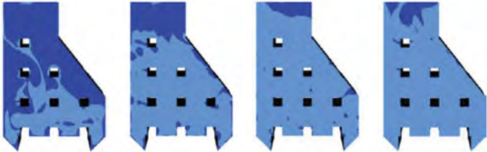
Figure 3 – End section of tee filling for \tau_0 = 25 Pa, \tau_0 = 12.5 Pa, \tau_0 = 5 Pa and \tau_0 = 1.0 Pa.
