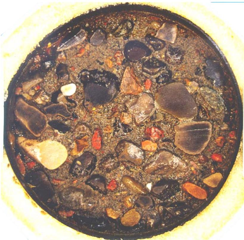
Image of sample taken from the top of the cylinder, showing severe scaling, with completely exposed aggregate particles to a depth of several mm.
