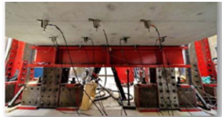
*Fig.4: Bottom view slab with acoustic emission sensors*
