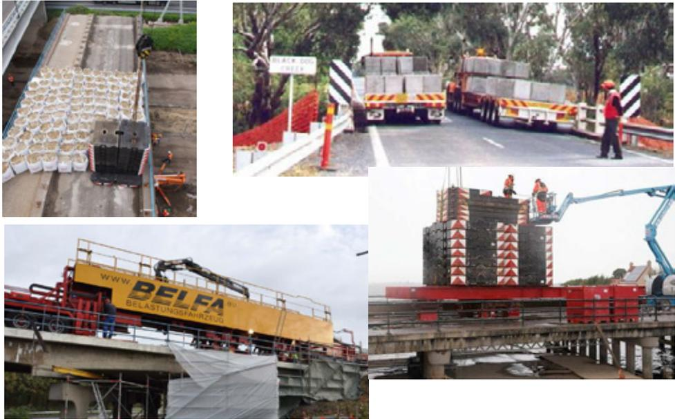
*Fig.5: Different setups proof loading slab viaducts*
