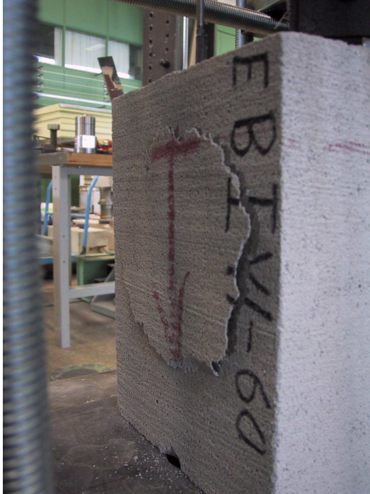
Figure 4. Cracking after 2 mm displacement in those specimen with eccentric reinforcement and without transverse force.
