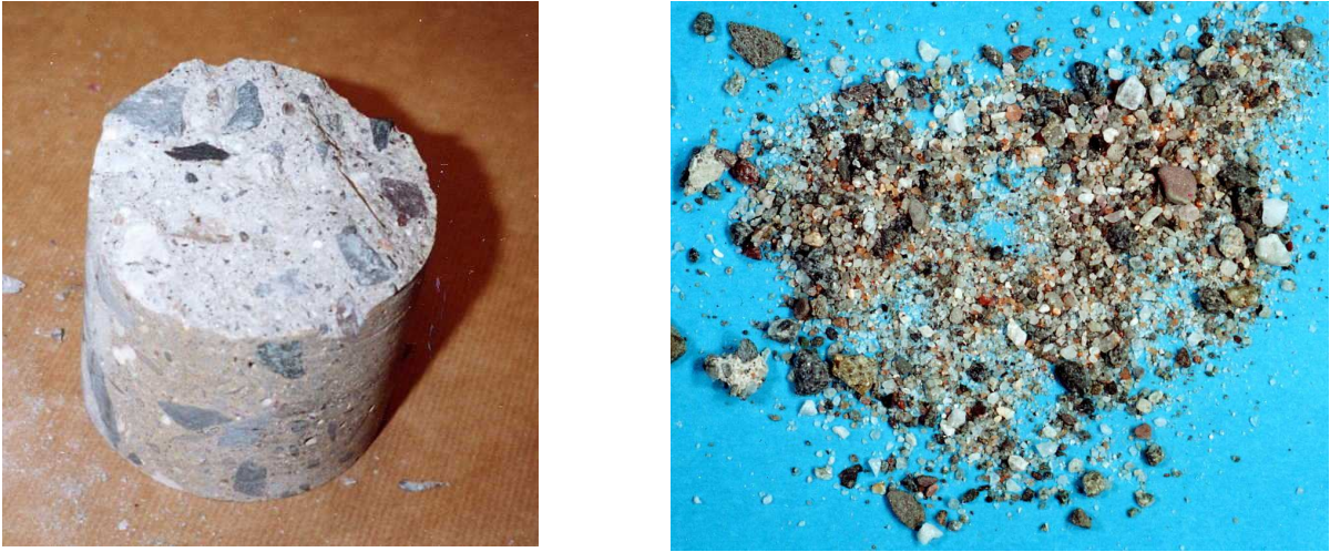
Figure 3 – Left: Part of a water-saturated concrete core before separation of the aggregate Right: The “concrete” after separation, but before washing in acid
