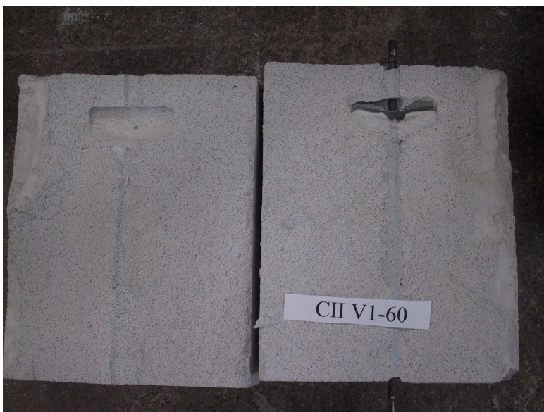
Figure 5. The corrosion protection coating (cement based) was broken when the test was stopped so that part of it was still attached to the AAC behind cross bar.
