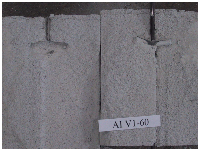
Figure 3. Bending of a 60 mm long cross bar when the test was stopped.
