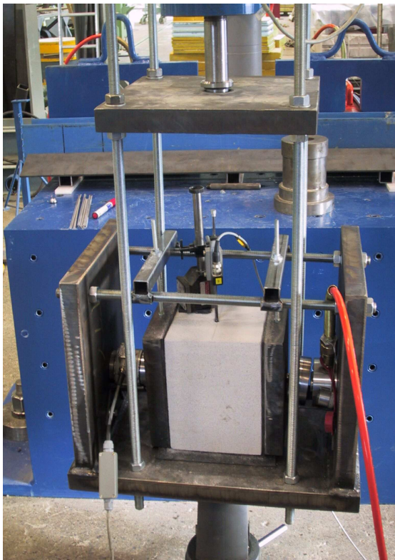
Figure 1. Test rig for pull-out tests.
