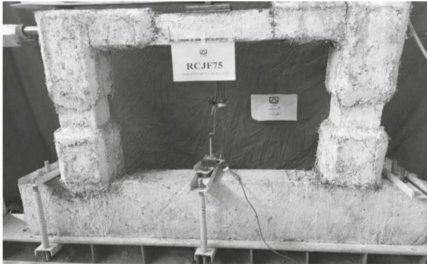
*Figure 3 – Initially damaged frame strengthened with HPFRCC (RCJF75) before testing.*
