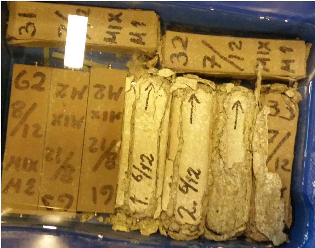
Figure 3 – Condition of mortar prisms stored in 5%  $\text{Na}_2\text{SO}_4$  solution for 2 years at 5°C. The light grey, deteriorated (spalled) prisms are the reference with 100% OPC. The brown ones marked M1 and M2 are mortar prisms where 20 and 35 vol% cement is replaced with calcined marl, respectively.
