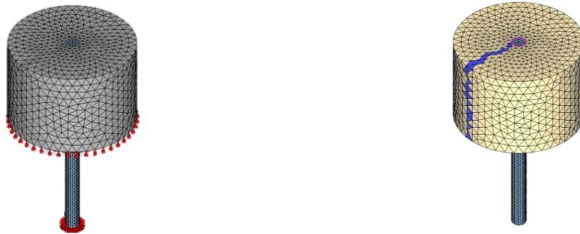
*Figure 2 – FE model of the specimens (left) and cracked elements (right)*
