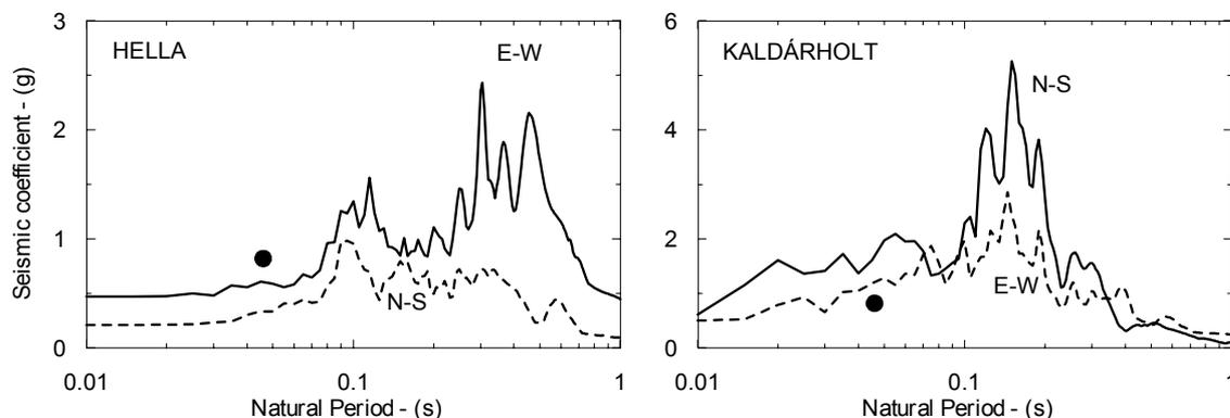
Figure 11 - Linear elastic response spectra with 2% damping ratio at Hella and Kaldárholt, based on the South Iceland earthquake of June 17, 2000. Both the horizontal components are shown. The dot shows the crack point for the shear wall in Figure 6.
