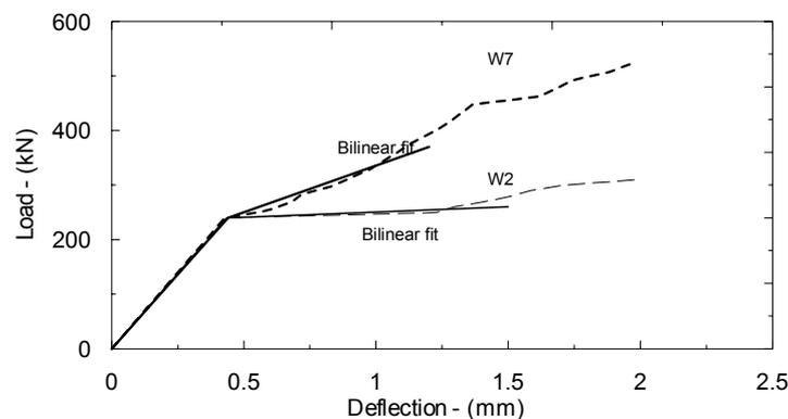
Figure 13 - Capacity curves for shear walls W2 and W7 from Figure 7 fitted with bilinear curves.
