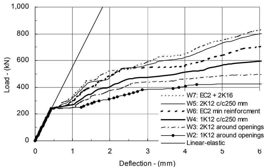
Figure 7 - Capacity curves for the shear wall with varying reinforcement.
