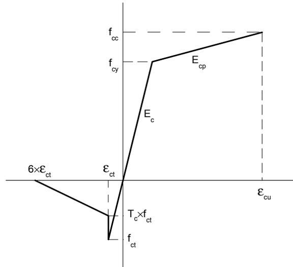
Figure 2 – Uniaxial concrete material model.
