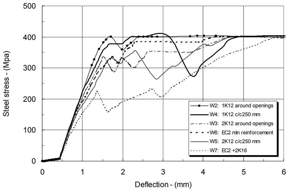
Figure 9 – Computed steel stresses at point A in Figure 6 for different reinforcement configurations as a function of deflection.
