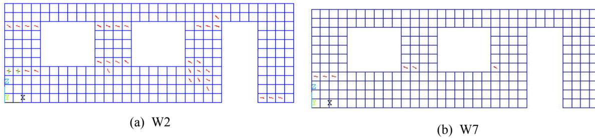
Figure 8 - Initial cracking in wall W2 and W7 at a load of 250kN.
