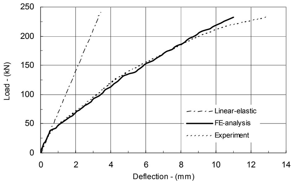
Figure 3 - Comparison of experimental [7] and FE-analysis [1] load-deflection curves for simply supported beam with shear reinforcement.
