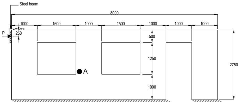
Figure 6 – Wall geometry used in pushover analysis. The reinforcement configuration is defined in Table 1. The dot to the right of the right window shows the location where the steel stresses are computed, in the diagram shown in Figure 9.
