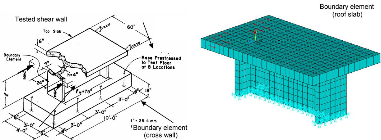
Figure 4 – a) Tilt-up of laboratory tested shear wall with boundary elements, from [8]. b) FE-model of the laboratory test from [1].
