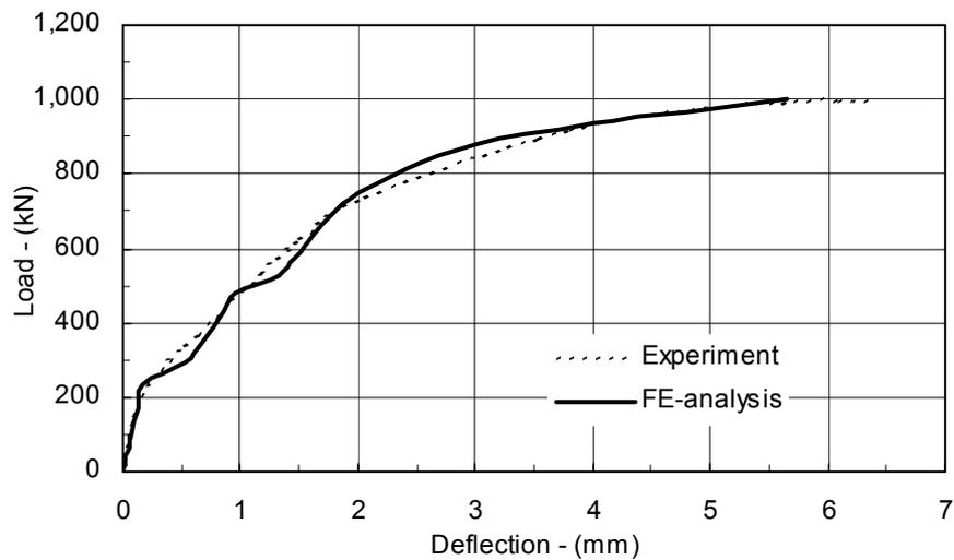
Figure 5 - Comparison of experimental [8] and FE-analysis [1] load-deflection curves for reinforced concrete shear wall with boundary elements.
