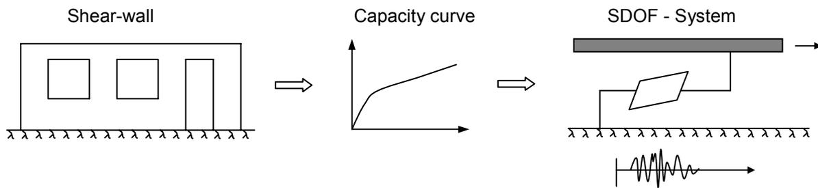
Figure 10 – Non-linear SDOF model of the shear walls, using the capacity curves to define the skeleton of the hysteresis rule.
