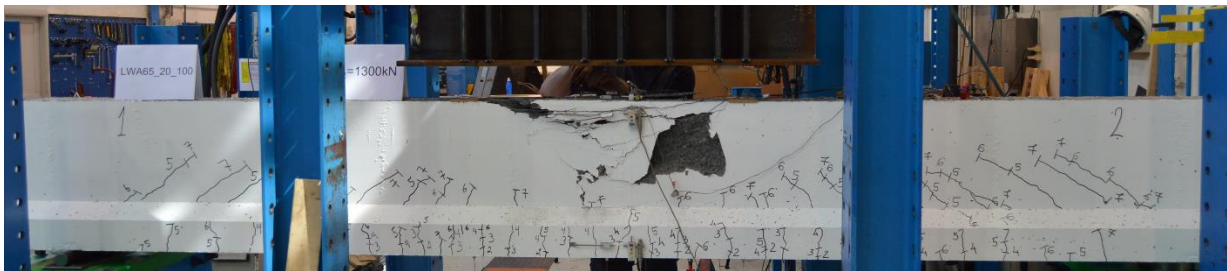
Figure 2– Final failure state of beam 4
