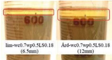
Figure 6 – Visible bleeding was observed for the matrices with filler and 0.18% LS.
