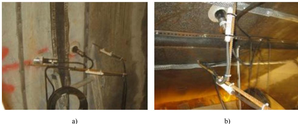
Figure 15 – Photos of strain gauges that failed during the third grouting, a) strain gauge ST23 and b) ST25. Also seen in the photo: the installed joint meters, a) JM01 and JM02 and b) JM03 and JM04.
